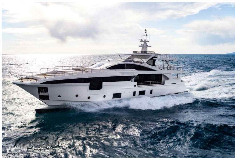
The Azimut Grande 35 Metri has a wave-piercing hull, extending the waterline as the bow rises out of the water
